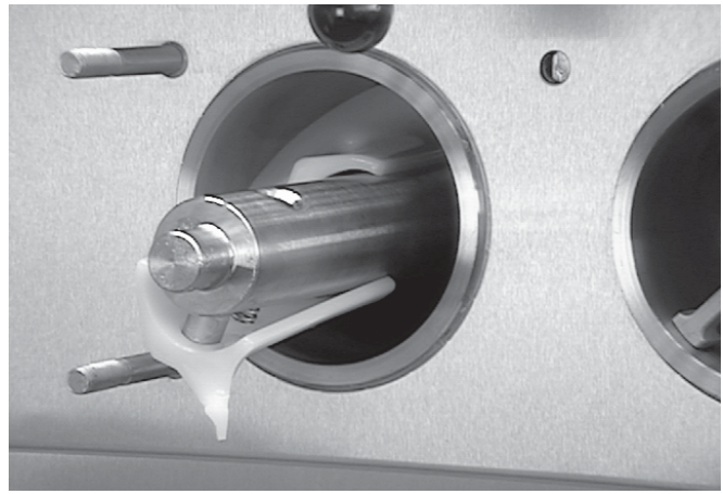
Figure 18. Auger Flight Removal
